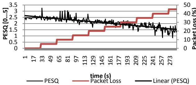
Figure 3. Calibration PESQ vs. Packet Loss
